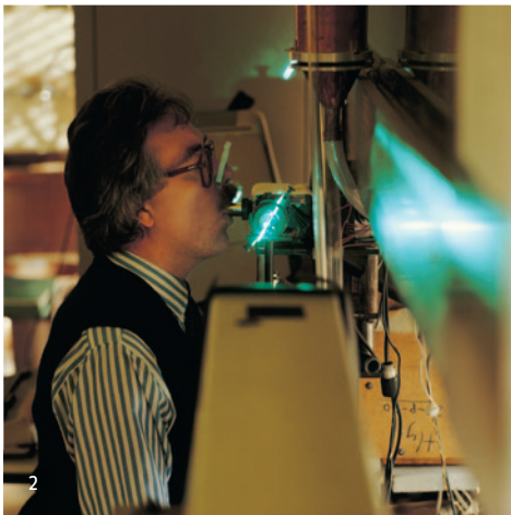
1 New building for the Computing Center and the Institute of Medical Informatics and Systems Research 2 Inhalation device for determining the particle deposits in the lung 3 Tests for the gas emission of timber preservatives into ambient air 4 Archiving of bio samples in the environmental specimen bank 5 Stele by Ben Muthofer in front of the Institute of Medical Informatics and Systems Research 6 Sculpture by Jochen Scheithauer at the main entrance road to the campus 7 Institute of Toxicology
