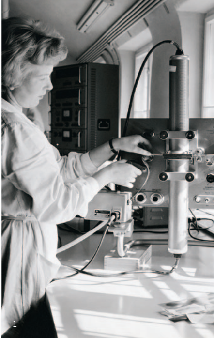
1 Teaching requisite qualifications in radiation protection: A course participant in front of a radio paper chromatograph 2 Test set-up at the Institute of Radiation Protection 3 Electron microscope at the Institute of Hematology 4 At the Institute of Radiation Protection, course participants have been taught in practical matters of radiation protection since 1960 5 Maintenance and storage facility and district heating station 6 Building site of the nuclear biology area, overlooking the administration building in the background 7 Facade of the lecture building for the Institute of Radiation Protection
